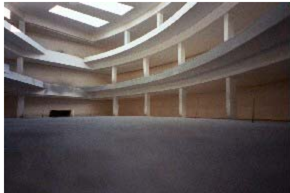
Fig. 1: Six well skylight model interior view looking north on a simulated June morning (note sunpatch on upper left). The skylights are evenly disposed somewhat to the east of the long axis (north-south) of the atrium
