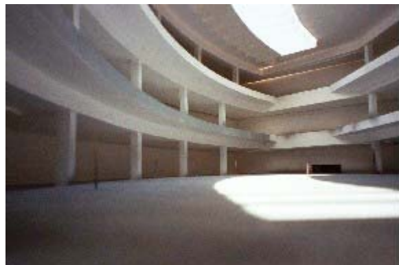
Fig. 2: Louvered skylight model interior view looking south at simulated June midday
