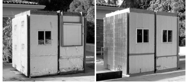
Fig. 2: The experimental and control cells viewed from the south with the shade system and without the shade system
