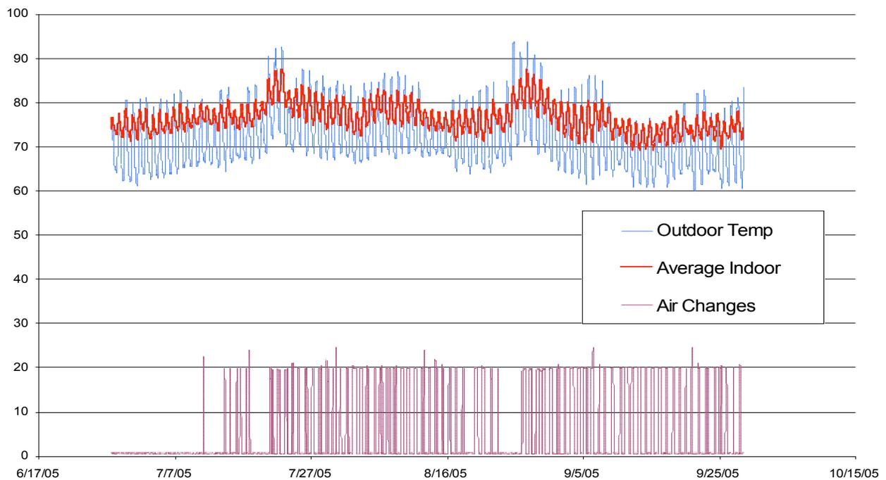
Fig. 3: The Second Floor low-mass unit with the attic shows much greater diurnal change in Average Indoor Air Temperature compared to the first floor unit. This second floor unit also experienced higher peak indoor temperatures in spite of regular use of the whole house fan. However at night minimum temperatures were always much cooler than the first floor unit. (Note the heat wave between August 22 to September 3 is analyzed in more detail in Figs 4 to 6 below.)
