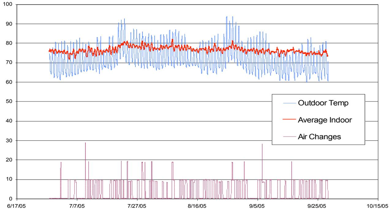
Fig. 2: The First Floor slab-on-grade unit shows very little change in Average Indoor Air Temperature compared to Outdoor Air Temperature. The spikes in Fan Power indicate that occasionally the owner also turned on the furnace fan to help circulate air in addition to the whole house fan. Note that the indoor air temperature exceeded 80°F on only three days
