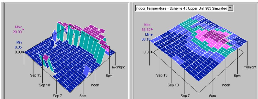
Fig.5 During the design phase HEED predicted that the peak Indoor Air Temperature (right) would be 86.82°F in the low mass upper unit. The ventilation patten for the 20 Air Change whole house fan (left) needed only a few hours each night to being minimum indoor temperatures down to the high 60's, which was below the bottom of the comfort range.
