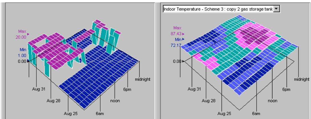
Fig.6 The recorded data in this same upper floor unit shows that the occupants experienced a peak Indoor Air Temperature of 87.43°F (right), which is within 1 degree of HEED's predicted peak temperature (see Fig.5). Note that the occupants did not use their whole house fan during the first day of the heat wave, and two days later they kept the fan running during the increasing heat of midday (left).
