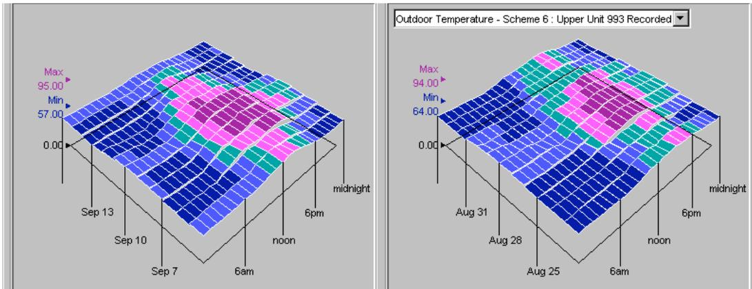
Fig.4 The peak Outdoor Air temperature recorded on site was 94°F (right) between August 22 through September 3. In order to compare this actual performance with HEED's predictions during the design phase, using EPW climate data for this climate zone a similar temperature pattern was found that peaked at 95°F between September 4 through 15 (left).
