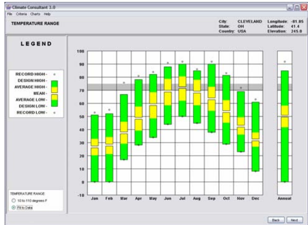
Fig.1: This Temperature Range Chart is the simplest of all charts, in this case showing dry bulb temperatures for Cleveland for all 12 months and also for the full year.
